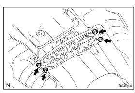
15. REMOVE 4 ENGINE REAR MOUNTING SET BOLTS
