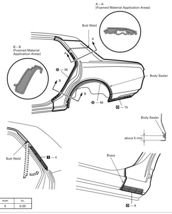
Before temporarily installing the new parts, apply body sealer to the wheel arch.
