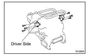
(c) Remove the 3 screws and the servomotor.
