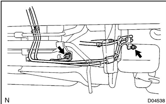
(b) Install the oil cooler pipe with 2 nuts.
