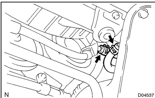
(c) Connect the 2 hoses and clamp the 2 clips.
