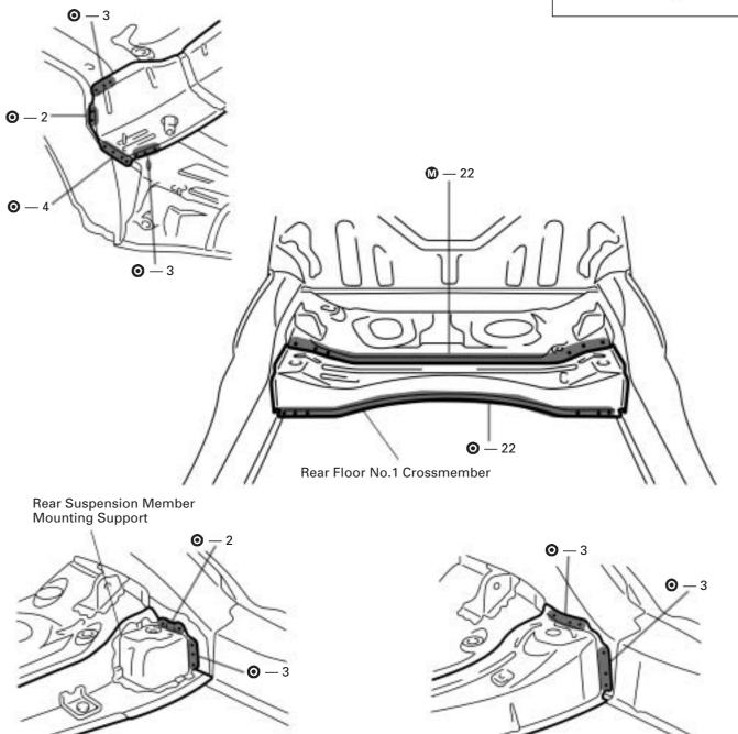
1. After removing the rear floor No.1 crossmember, disconnect the welding between the rear suspension member mounting support and the rear floor side member.
