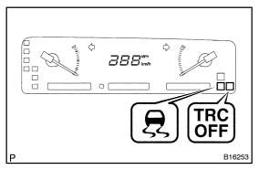
(4) Press the TRC OFF switch again to change the TRC system to operational condition and check that the TRC OFF indicator light goes off.
