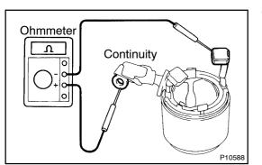
7. INSPECT FIELD COIL FOR OPEN CIRCUIT
