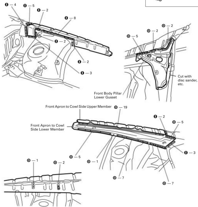
After removing the front body pillar lower gusset and front apron to cowl side lower member, remove the front apron to cowl side upper member.
