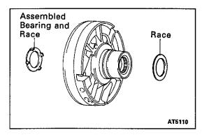
(d) Remove the assembled bearing and races from the overdrive support.
