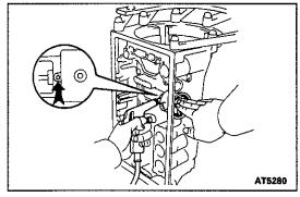
(b) Applying compressed air to the oil hole, remove the second cost brake cover, piston assembly and spring.
