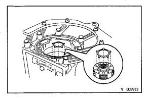
(c) Remove the race from the front planetary gear.
