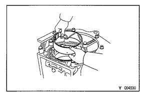
(c) Remove the second coast brake band from the case.HINT: For the method of inspection.(See page AT-37)
