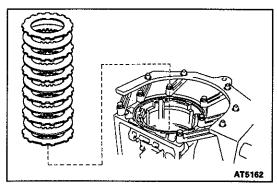
(b) Remove the flange, 5 plates and 5 discs as a set.
