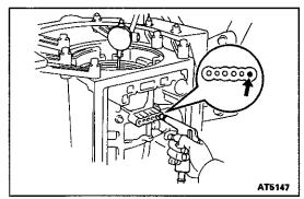
(b) Measure the stroke applying and releasing the compressed air (392-785 kPa, 4-8 kgf/cm² or 57-114 psi), as shown.
