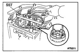
(c) Using SST, remove the overdrive support assembly. SST 09350-30020 (09350-07020)
