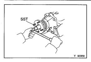
(b) Using SST, remove the nut. SST 09060-20010
