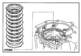
(b) Remove the 1 flange, 5 plates and 5 discs.
