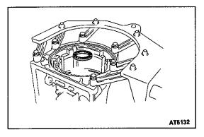
(d) Remove the bearing from the first and reverse brake.
