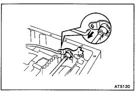
(b) Disconnect the parking lock rod from the manual valve lever.
