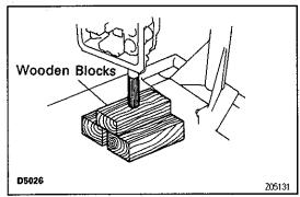
(d) With wooden blocks under the output shaft, stand the transmission on the output shaft.
