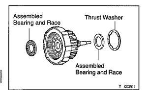
(c) Remove the assembled bearing and race, thrust washer and race from the forward clutch.
