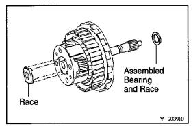
(b) Remove the race and assembled bearing and race.
