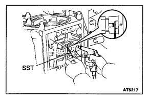
(b) Using SST, measure the stroke applying the compressed air (392-784 kPa, 4-8 kgf/cm² or 57-114 psi), as shown.
