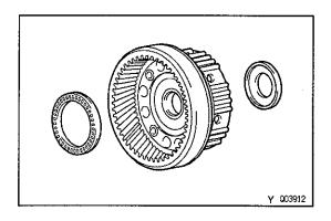
(b) Remove the bearings and race from the front planetary ring gear.
