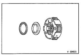
(b) Remove the bearing and race from the front planetary gear.
