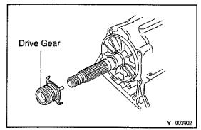
11. REMOVE SPEEDOMETER DRIVE GEAR AND SENSOR ROTOR
