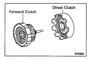
(b) Remove the direct clutch from the forward clutch.
