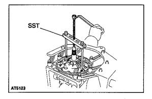
(b) Using SST, remove the oil pump. SST 09350-30020 (09350-07020)
