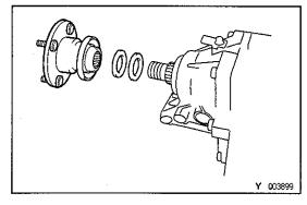
(c) Remove the output flange and 2 washers.
