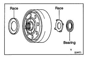
(b) Remove the bearing and races from the planetary ring gear.
