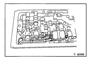
(b) Disconnect the 5 connectors from the solenoids.
