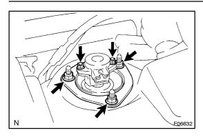
(c) Remove the 2 nuts and suspension control actuator.
