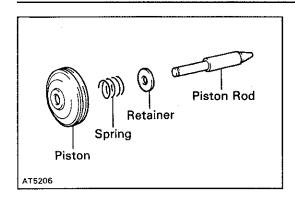
(c) Remove the compression spring, retainer and piston rod.
