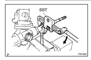
(b) Using a wrench, hold the steering rack steadily and using SST, remove the rack end.
