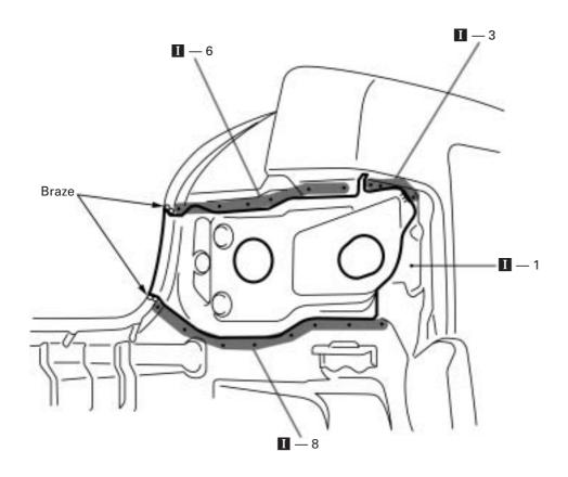
Temporarily install the new part and check the fit of the luggage compartment door and rear conbination light.
