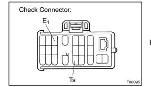
(3) Using SST, connect the terminals Ts and E<sub>1</sub> of the check connector.
