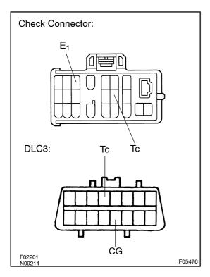
(6) Using SST, connect terminals Tc and E<sub>1</sub> of the check connector or Tc and CG of the DLC3.
