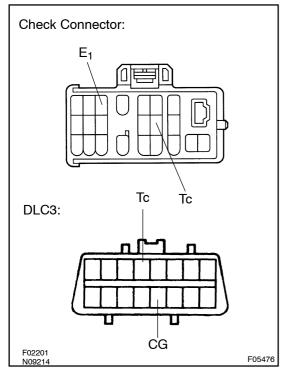
(2) Using SST, connect terminals Tc and E<sub>1</sub> of the check connector or Tc and CG of the DLC3.
