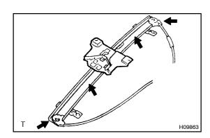
(1) Apply MP grease to the glass guide and rollers of window regulator.
