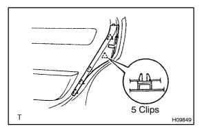
**20. INSTALL SIDE TRIM BOARD REAR NO.2 COVER** Install the side trim board rear No.2 cover.
