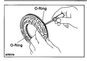
(d) Using a small screwdriver, remove the 2 O-rings from the piston.
