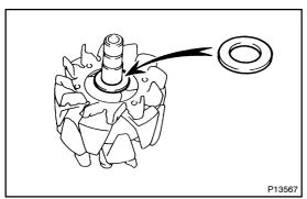
(c) Place the bearing cover (inside) on the rotor.
