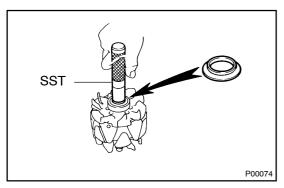
(e) Using SST, push in the bearing cover (outside). SST 09285-76010
