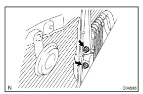
(b) Remove the 2 nuts and oil cooler.
