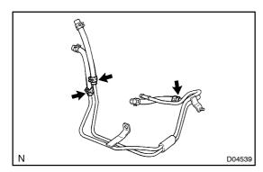
(c) Loosen the 3 clips and disconnect the 3 hoses.
