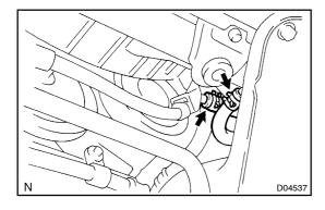
3. REMOVE OIL COOLER PIPE(a) Loosen the 2 clips and disconnect the 2 hoses.
