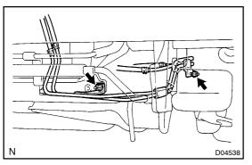
(b) Remove the 2 nuts and oil cooler pipe.
