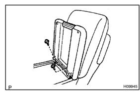
**21. REMOVE REAR CONSOLE ARMREST** Remove the 2 screws and rear console armrest.
