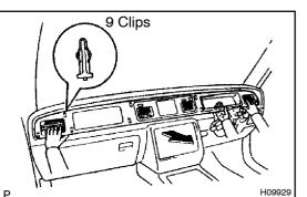
7. **REMOVE CLUSTER FINISH PANEL ASSEMBLY** Remove the cluster finish panel assembly as shown in the illustration.
