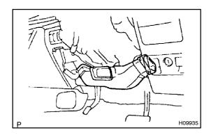
**12. REMOVE NO.2 HEATER TO RESISTER DUCT** Remove the No.2 heater to resister duct.
