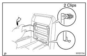
**25. REMOVE NO.2 CONSOLE REAR END PANEL** Using a moulding remover, remove the No.2 console rear end panel.
