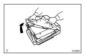
(e) Remove the center seatback cover as shown in the illustration.
