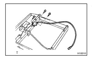
(h) Remove the 3 screws and limit switch.
