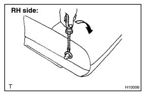
(d) Using a screwdriver, remove the seatback protector shaft bushings.
