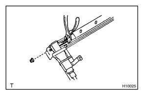
(b) Using pliers, hold the horizontal jack screw and remove the nut.
