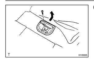
(c) Remove the screw and seatback lock cover as shown in the illustration.
