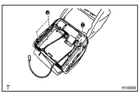
(f) Remove the 4 nuts and front seatback foot rest frame.
