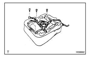
**18. INSTALL FRONT SEAT CUSHION ASSEMBLY** Install the front seat cushion assembly with the 4 bolts to the seat adjuster.
