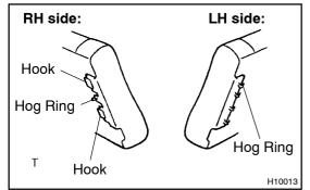
(b) Install new hog rings at position as shown in the illustration.
