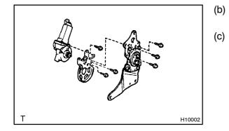
Install the motor bracket with the 3 screws to the power
