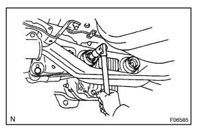
(b) Using a 12 mm hexagon wrench, remove the 2 bolts.
