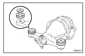
(d) Remove the adjusting shims and upper mount stoppers from the differential carrier.
