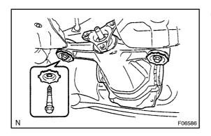
(c) Remove the 2 bolts, lower mount stoppers and differential carrier.
