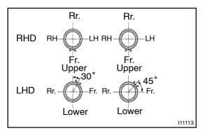
Install the hose clip in a position, as shown in the illustra-
