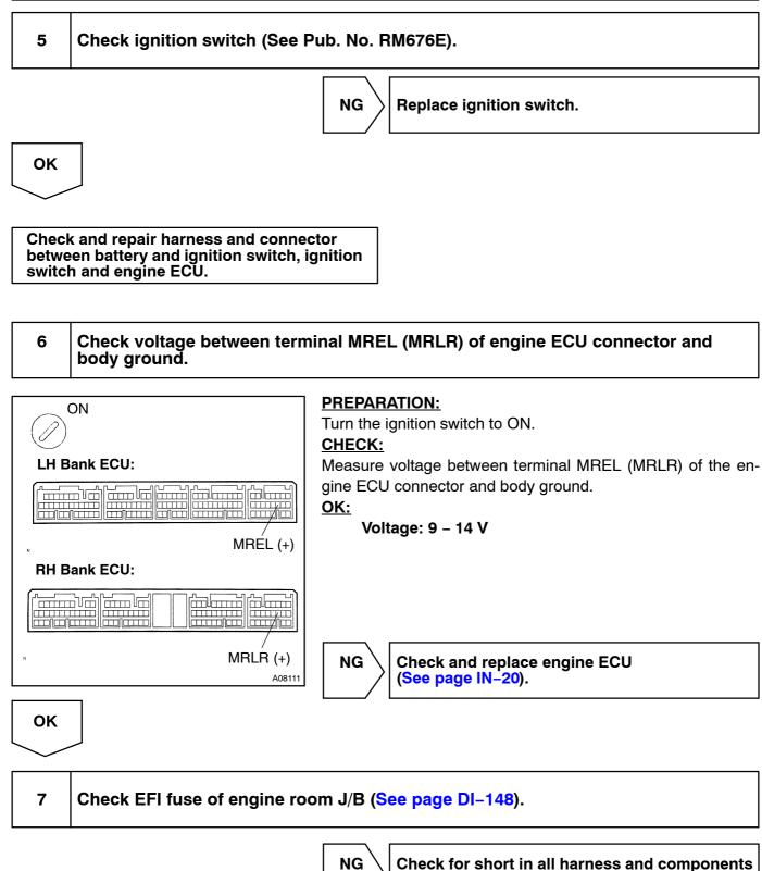
connected to EFI fuse.
