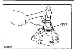
2. INSTALL OIL SEAL TO EXTENSION HOUSING
