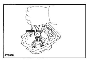
(b) Using a snap ring expander, install the snap ring.
