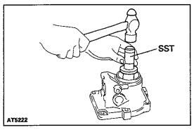
(b) Using SST, drive out the bearing. SST 09325-12010
