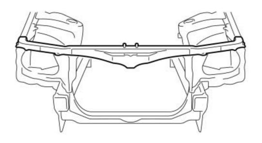
Temporarily install the new parts and measure each part in accrodance with the body dimension diagram.
