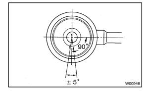
(b) Using SST and a press, install a new cushion as shown in the illustration.
