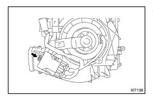
4. INSTALL BLOWER MOTOR CONTROL RELAY Install the blower motor control relay with the screw.
