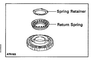
(c) Remove the spring retainer and return spring.
