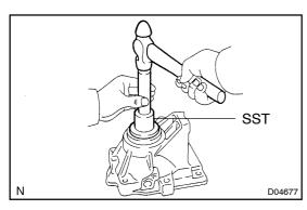
2. INSTALL OIL SEAL TO EXTENSION HOUSING Using SST and a hammer, install a new oil seal. SST 09517–12010
