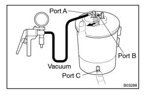
(b) Apply vacuum (1.96 kPa (20 gf/cm², 0.28 psi)) to port A, check that the vacuum does not decrease when port B and C are closed, and check that the vacuum decreases when port B is released.
